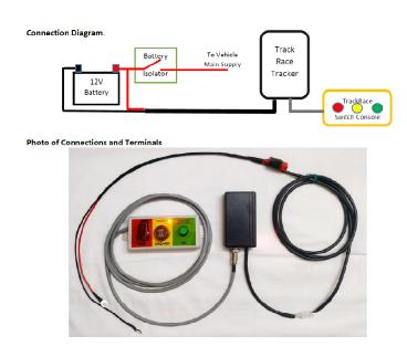
A minimum of 100mm of Track Race Power Supply Cable and Console cable should be left at the unit mounting location for connection to the unit.
